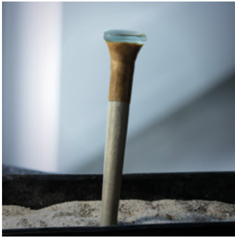
The pre-shaped rough stone is cemented on the putty rod.
